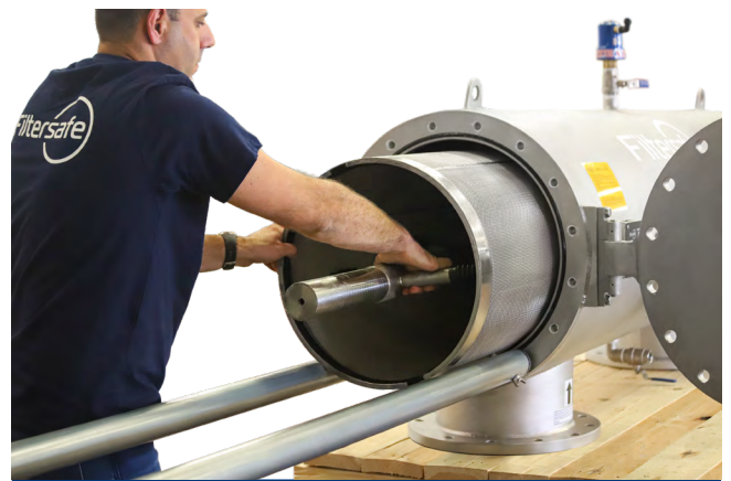
The TITAN Incorporates Smart Design for Easy Maintenance
