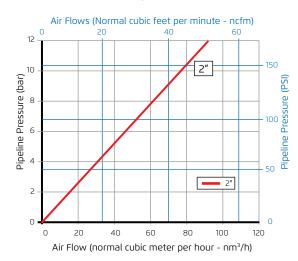
Air relief and intake charts are based on actual measurements, made in Bermad Air Flow test bench, according to EN-1074/4 standard and refer to Side outlet.
