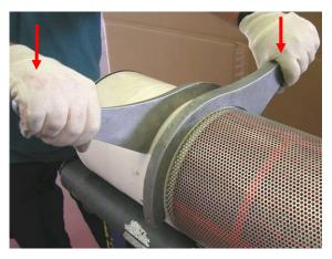
Insert the fine screen back to the filter housing (A). Use the fork part of the Push Pull Tool to lift the screen and push it through the last few centimeters till it is correctly seated in the filter housing (B).
