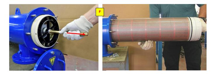
6. Depending on the actual diameter of your filter use two units of Amiad's Screen Separation Tool (Catalog Number 700190-001985 for 2"-8" , 700190-002139 for 10"-12" or 700190-002150 for 14"-16" filters) to separate the Chamber Flat Screen and the Dirt Collector from the Fine Screen.
