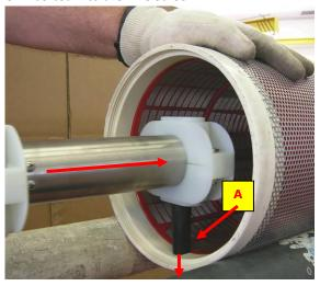
2. Use the two Amiad's Screen Separation Tools to reconnect the Chamber Flat Screen and the Fine Screen.
