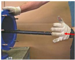
4. Insert the Coarse Screen back to the filter housing (A), return the filter's lid back to its closed position (B) and retighten the lid bolts nuts (C).
