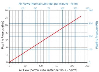
Air relief and intake charts are based on actual measurements, carried out in Bermad Air Flow test bench, according to EN-1074/4 and AS4883 standard and refer to Side outlet. Use Bermad Air software for optimized Sizing & Positioning of Air Valves. Model C80
