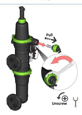
c. Push out the actuator valve as shown below
