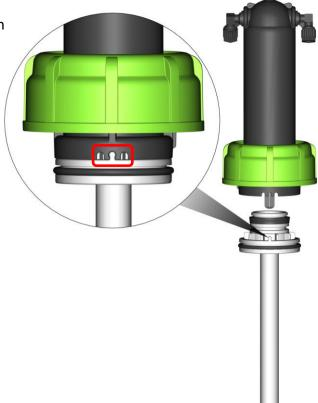
b. Insert the cylinder assembly to the cover, ensuring that the key shaft was inserted in the right
