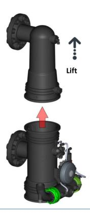
The installation configuration can be changed by rotating the lower body  $0^{\circ}$  -  $360^{\circ}$
