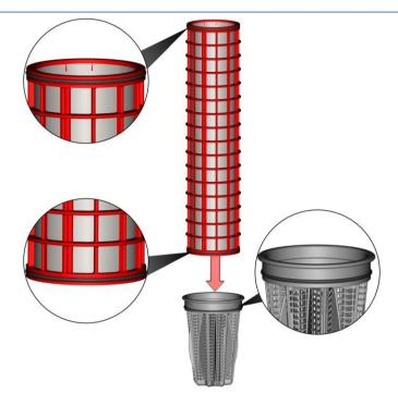
2. Insert the scanner into the fine and coarse screen
