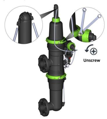
c. Remove both clamps (hold the filter cover while removing the clamps)
