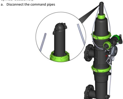
b. Open the nut using the Sigma multi-tool
