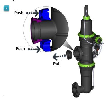
3. Remove the flange from the Sigma body
