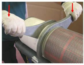
3. Insert the fine screen back to the filter housing (A). Use the fork part of the Push Pull Tool to lift the screen and push it through the last few centimeters till it is correctly seated in the filter housing (B).
