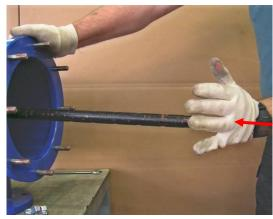
Insert the Coarse Screen back to the filter housing (A), return the filter's lid back to its closed position (B) and re-4. tighten the lid bolts nuts (C).
