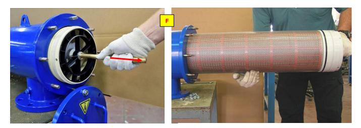
6. Depending on the actual diameter of your filter use two units of Amiad's Screen Separation Tool (Catalog Number 710103-001455 x 2) to separate the Chamber Flat Screen and the Dirt Collector from the Fine Screen.
