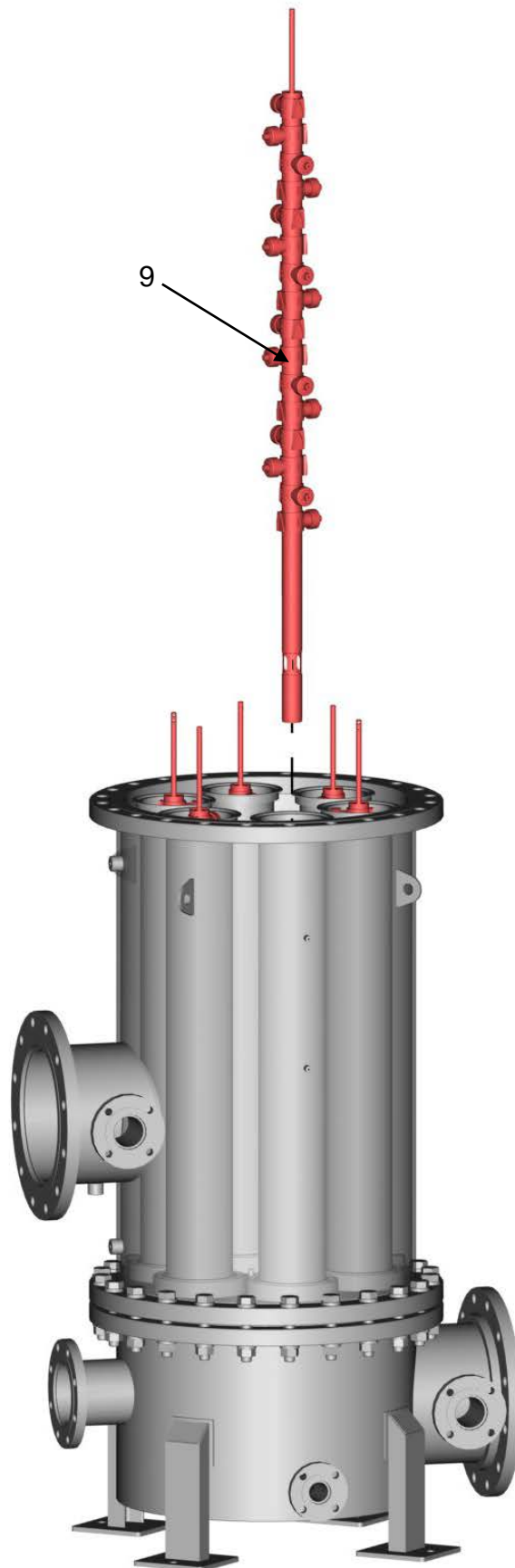
Figure 13 - Suction Scanner Removal
