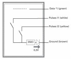
\* active for HRI Data Unit only External power supply of 5 to 24 V DC possible if data line is not used (green)
