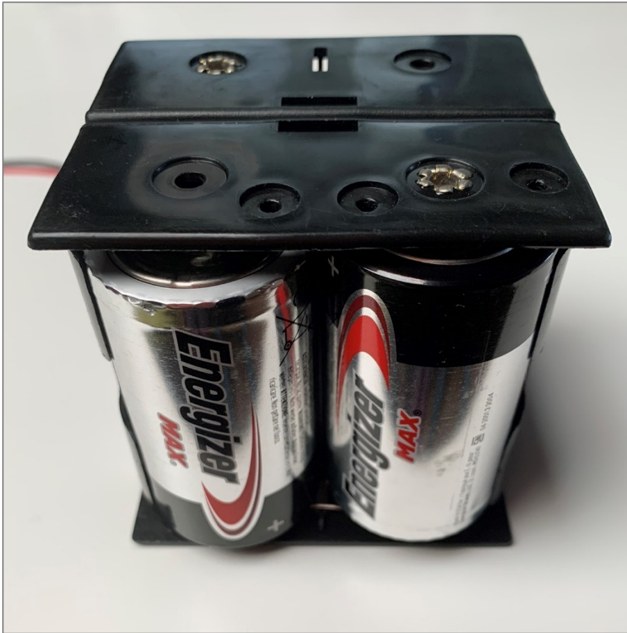
Figure 12: Battery assembly with 4 x 1.5V D batteries
