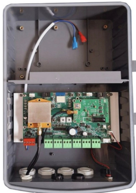
SAPIR 2 MINI DC - 6 OUT / 4 IN / 2 ANA IN + 4G Cellular Modem + RF G5 MASTER Interface
