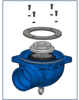
Figure 12 - Replacing the seals - B
