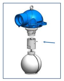
Figure 32 - Reassembling - H
