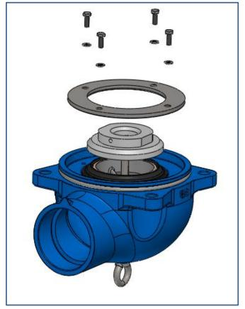
Figure 20 - Replacing the seals - D
