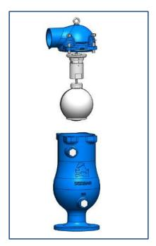
Figure 33 - Reassembling - I
