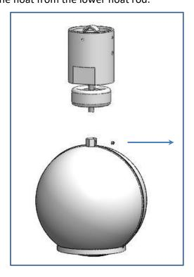
Figure 15 - Disassembling the air valve - B
