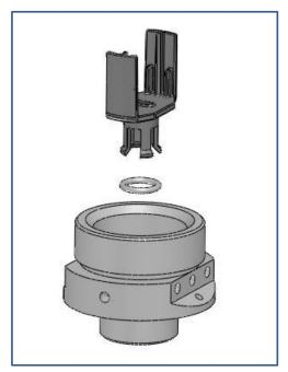
Figure 19 - Replacing the seals - C
