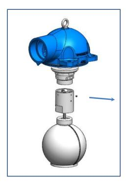
Figure 14 - Disassembling the air valve - A
