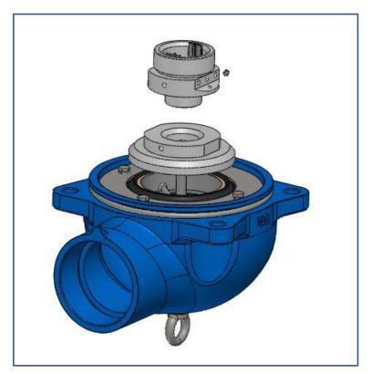
Figure 18- Replacing the seals - B
