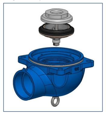
Figure 21 - Replacing the seals - E
