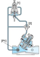
The Pressure Sustaining Pilot [1] commands the main Valve to throttle closed should Upstream Pressure [P1] drop below setting, and to open fully when [P1] rises above setting. The Manual Selector [2] enables local manual closing.
